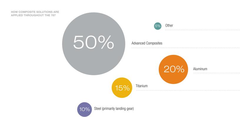
In addition to lowering the overall airplane weight, moving to a composite primary structure promises to reduce both the scheduled and nonroutine maintenance burden on the airlines.
