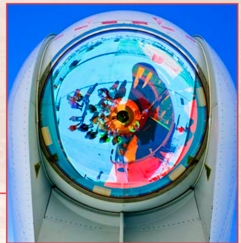
PHOTOS: (Left) The Airborne Laser Test Bed, a modified 747-400, flies over Edwards AFB, Calif. U.S. AIR FORCE (Inset) The beam from the laser was directed through this optic in the aircraft’s nose. KURTISS HUMPHREY/BOEING
