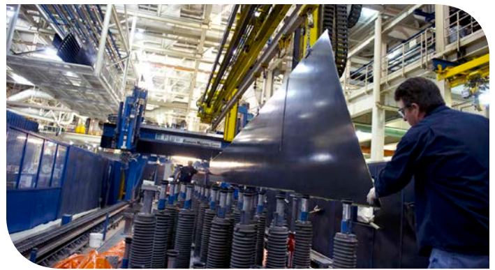
PHOTOS: (Clockwise from far left) Boeing manufacturing sites collect excess carbon fiber material for recycling. ALAN MARTS/BOEING Boeing South Carolina produces one-piece 787 composite fuselage barrels, known as the aft fuselage sections 47 and 48. ED TURNER/BOEING Richard Moore loads a composite skin panel onto an abrasive water jet trimming machine; mechanic Fred Staples measures fastener height on a 787 vertical fin; Composite Manufacturing Center employees prepare to load a completed 787 vertical fin onto a trailer for shipping. BOB FERGUSON/BOEING
