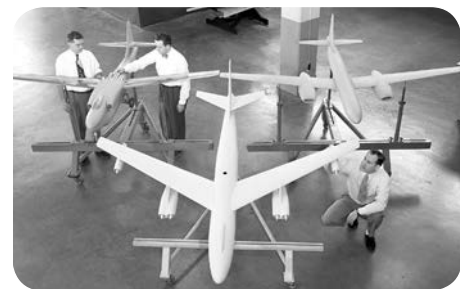
PHOTO: These models show the evolution of the B-47 design from a conventional straight-wing airplane to a radical swept-wing bomber with innovative podded engines. BOEING ARCHIVES
