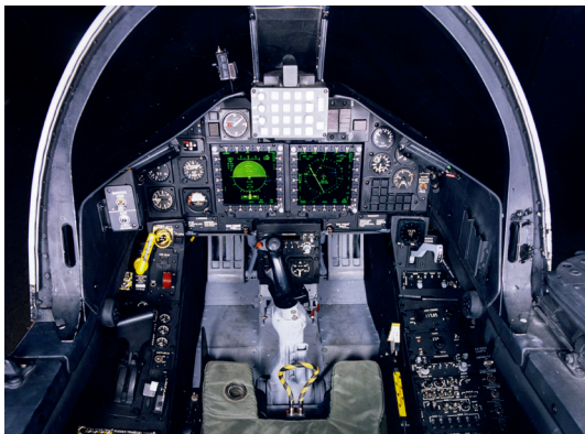
PHOTOS: (Clockwise from far left) The T-45A Goshawk jet trainer is at the heart of the T45TS, the U.S. Navy's first totally integrated training system for undergraduate jet flight training; the T-45C's digital cockpit resembles that of a front-line U.S. Navy fighter such as the F/A-18 Super Hornet; the T45TS includes advanced flight simulators. BOEING ARCHIVES
