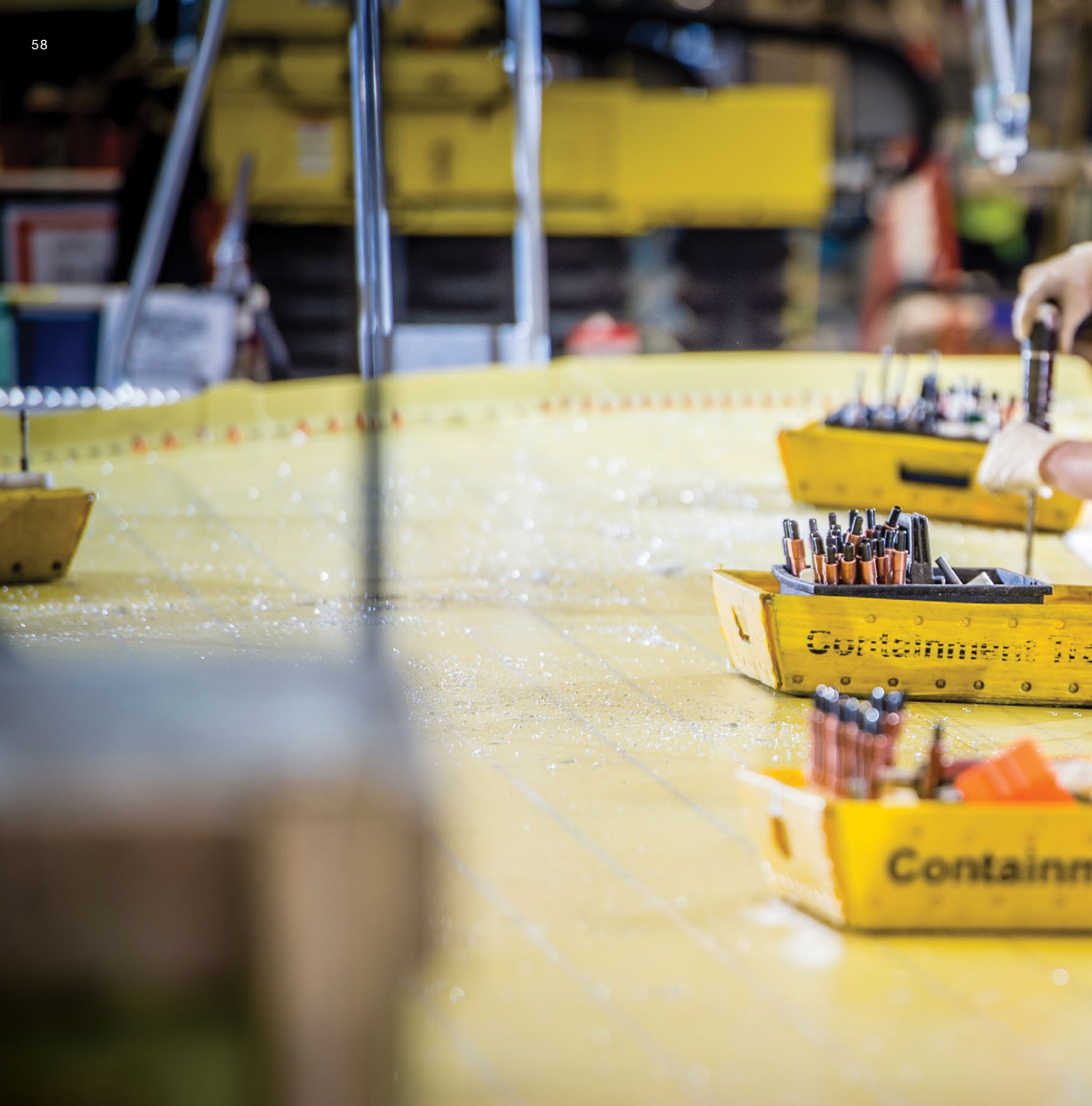
Employees drill holes in the top panel of a 737 wing in Renton, Wash., before installing fasteners.
