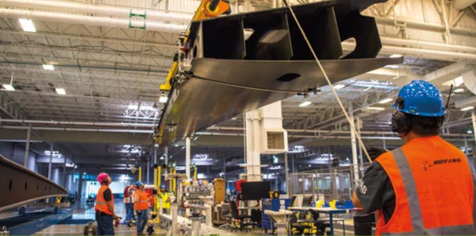
Photos: (Above) Assisted by a crane, employees in West Jordan move a 787 horizontal stabilizer. (Below) Mike Thomas, left, and Jacob Cleland guide it into place.
