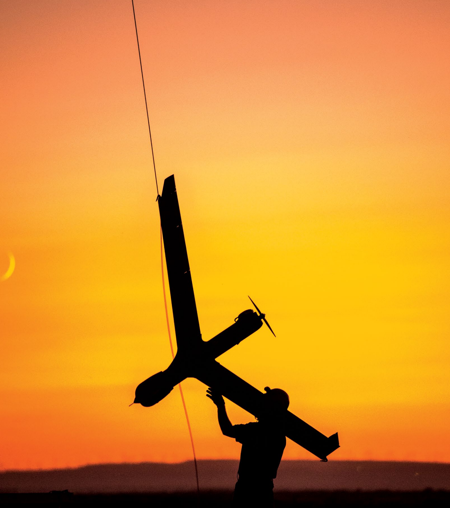
Photos: (From left) A flight operations team member untethers ScanEagle from a 300-foot-long (100-meter) cable used by FLARES to capture it; FLARES hovers over the Oregon landscape carrying a static weight.
