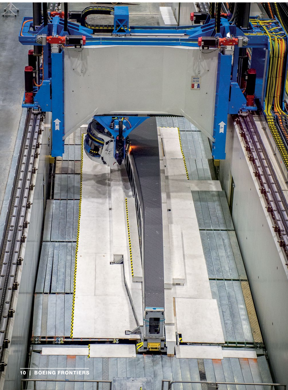
Photos: (Above) A spar-lamination machine will be used to make 777X wings out of carbon-fiber material in Everett. (Left) The machine will lay carbon fiber on a form, which will then be baked inside an autoclave, creating parts for a 777X wing at the Composite Wing Center.
